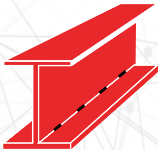
H-beam assembling (by auto Spot Welding)
